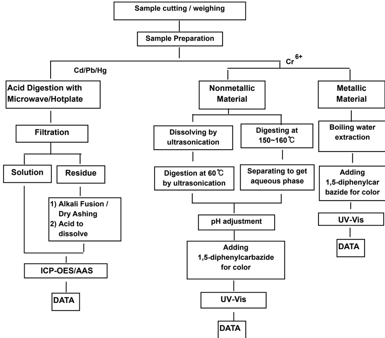
The samples were dissolved totally at the acid digestion step of the above flow chart for Cd,Pb,Hg
